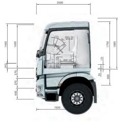
Engine tunnel: 170 mm Standing headroom on engine tunnel: 1460 mm
