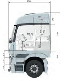
Engine tunnel: 170 mm Headroom on engine tunnel: 1785 mm Headroom in front of the seats: 1840 mm
