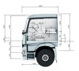
Engine tunnel: 170 mm Standing headroom on engine tunnel: 1460 mm
