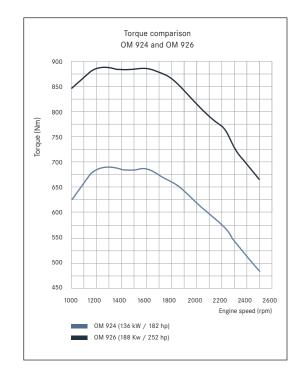
More power – less fuel. From 136 kW (182 hp) to 188 Kw (252 hp) the OM 92X engine series makes their maximum torque available in the lower, fuel-efficient engine speed range.
