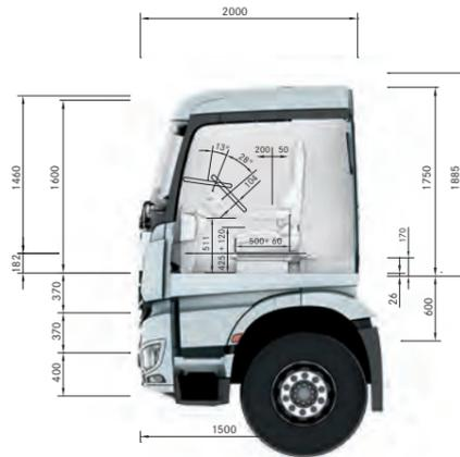
Engine tunnel: 170 mm
