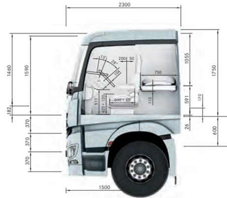
Engine tunnel: 170 mm
