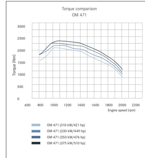
More power – less fuel. From 310 kW (421 hp) to 375 kW (510 hp) the OM 471 engines make their maximum torque available in the lower, fuel-efficient engine speed range.
