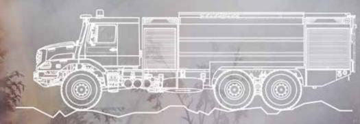
The position of the cab behind the front axle and the truck's suspension tuning provide an ideal off-road workplace in the Zetros.
